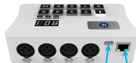
Universe #1,2,3,4 1 DMX1 ground 2 DMX1 data- 3 DMX1 data+
