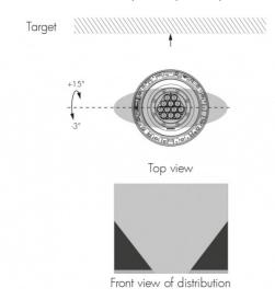
Vertical distribution :  $90^{\circ}x6^{\circ}$ ,  $90^{\circ}x15^{\circ}$ ,  $90^{\circ}x25^{\circ}$ ,  $90^{\circ}x35^{\circ}$
