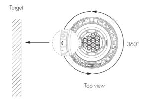
The optical chamber can be rotated until the arrow faces the target. Refer to the installation instructions for details.
